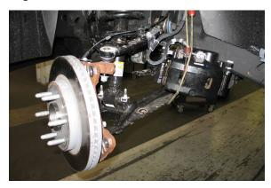
11. Remove the three 15mm bolts on the backside of the hub assembly, detach it from the steering knuckle.
