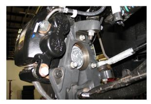
24. Attach the brake line and ABS line brackets, ABS sensor plug on the frame, and the hold down clips in their original locations.
