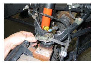
10. Remove the 18mm bolts holding brake caliper assembly from the steering knuckle. With a metal wire or bungee cord attach the caliper no the chassis to prevent damage to the brake line. Next, remove the brake rotor and set aside.
