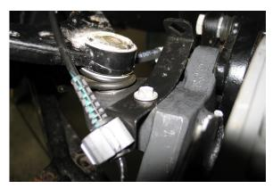
25. Rotate the spindle in both directions to confirm the brake line and ABS line have enough slack. If either is too tight, then you pull it through the bracket to give it the proper amount of slack.
