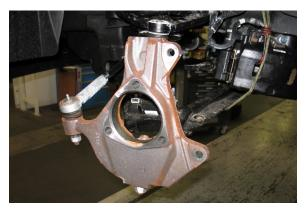
13. With a 18mm socket, break loose the upper ball joint nut but keep the nut partially threaded on the stud to keep the arm from swinging up and to keep it in place while removing the lower ball joint. Using a ball joint separator tool, free the upper ball joint from the steering knuckle.
